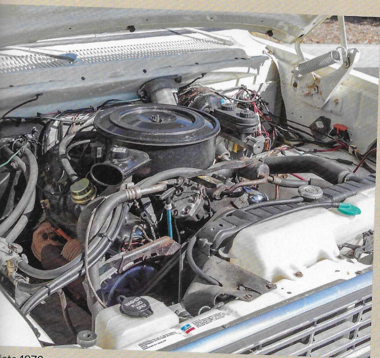
Late 1970s were a period when light-truck makers struggled to meet emissions requirements. The Palomino's cluttered engine compartment is full of hang-on smog equipment of the time.
